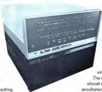
The *Altair 8800* includes the CPU board, front panel control board, power supply (enough to power any additional cards), and expander board (with room for 3 extra interface or memory modules) all included in a handsome, aluminum case complete with sub-panel and dress panel. Up to 16 cards can be added inside the main case.
