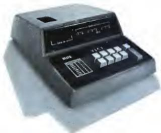
The Altair VLCT is ideal for machine language programming. It converts a three digit octal code directly into an 8 digit binary code for transmission to the computer and then displays the binary output from the computer in a 3 digital octal format. This allows you to program in octal which is much easier than programming in binary. In addition, the VLCT is much more convenient to work with than using the front panel switches of the Altair 8800.
