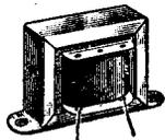
**filter condenser.** A condenser used in a filter system to permit passage of higher-frequency currents while limiting or blocking the flow of lower-frequency currents and direct current.
