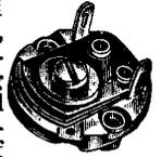
**triode.** A three-electrode vacuum tube, usually having a cathode, control grid and anode.
