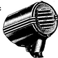
**Crystal Microphone.** A microphone depending upon the piezoelectric effect of Rochelle salt crystals to transform the mechanical stress produced by sound waves into electrical output. In general, crystal mikes are non-directional and have good frequency response.
