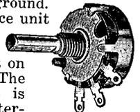
one end terminal. Rotating the movable contact thus varies the proportion of the total voltage which is transferred to the output circuit. The volume control of a receiver or p.a. amplifier is generally a potentiometer.
