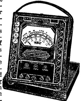
cuit for a particular measurement. Also known as a multitester, multiple-purpose tester or volt-ohm-milliammeter.
