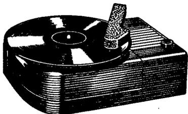
**record player.** A motor-driven turntable and a crystal or magnetic phono pick-up used for converting a phonograph record into audio frequency signals. These signals must be fed into the audio section of a radio receiver or into a separate audio amplifier for additional amplification before they can be reproduced as sound waves by a loudspeaker. When the amplifier and loudspeaker are built into the same cabinet with the record player, the combination is generally called an electric phonograph.
